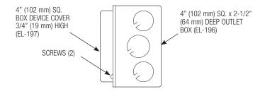
C Install Electrical Box into Wall Box as follows Assemble Mounting Bracket to Electrical Box using two (2) Screws (EL-125), internal tooth Lock Washers (EL-127) and Nuts (EL-126) provided.
