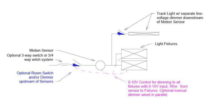
Lighting zones with lighting-devices and light-fixtures are indicated by wire lines and/or switch leg (SL) numbers.
