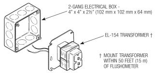
Note: One Sloan EL-154 transformer can operate up to ten OPTIMA equipped Flushometers. Run 18-gauge wire from transformer to Flushometer(s). Wire supplied by others. DO NOT supply power to transformer until installation of Flushometer is complete.
