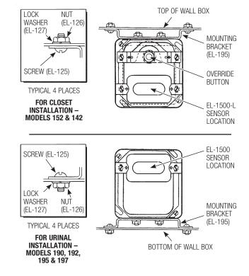
D Install Wall Box into wall in the exact location as illustrated in the Rough-in diagrams on Pages 2 and 3. Secure Wall Box using Drive Screws provided or other appropriate fasteners.
